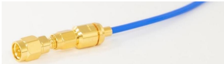
Figure 13 Cable to SSMA-SMA Adaptor Connection
