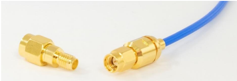
Figure 13 Disconnect the cable from SSMA-SMA Adaptor
