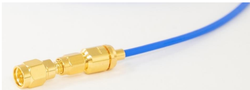
Figure 7 Cable to SSMA-SMA Adaptor Connection
