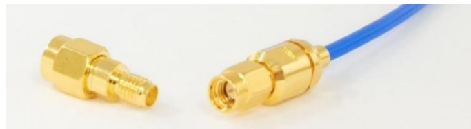
Figure 8 Disconnect the cable from SSMA-SMA Adaptor
