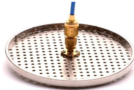
Figure 19 Connection to the connector at the ground plane of the discone
