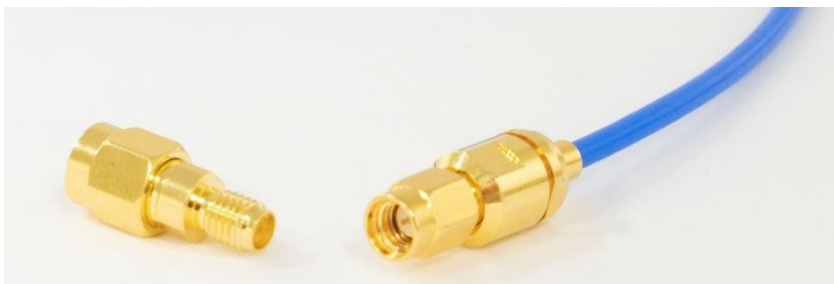
Figure 8 Disconnect the cable from SSMA-SMA Adaptor
