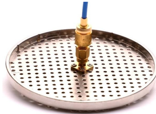
Figure 11 Connection to the connector at the ground plane of the monopole
