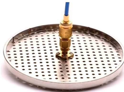
Figure 16 Connection to the connector at the ground plane of the monopole
