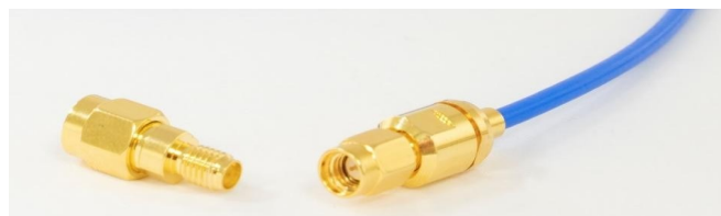
Figure 12 Disconnect the cable from SSMA-SMA Adaptor
