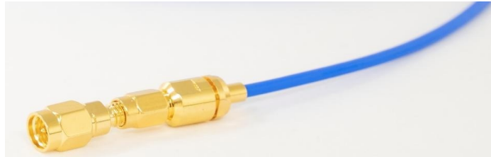
Figure 8 Cable to SSMA-SMA Adaptor Connection
