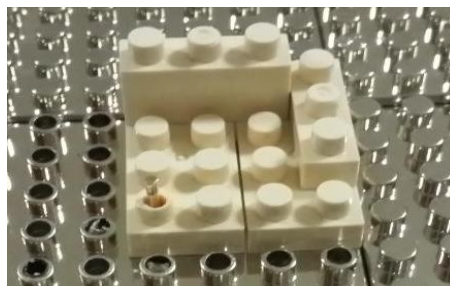
Figure 13 Dielectric cells above the ground plane
