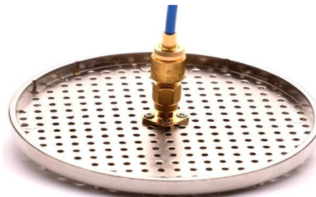
Figure 10 Connection to the connector at the ground plane of the monopole
