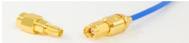
Figure 14 Disconnect the cable from SSMA-SMA Adaptor
