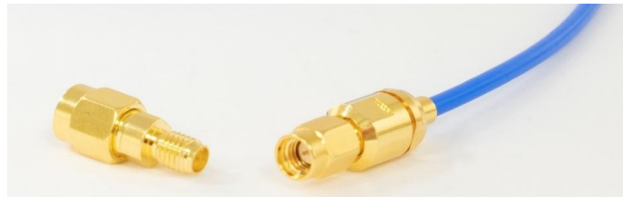
Figure 9 Disconnect the cable from SSMA-SMA Adaptor
