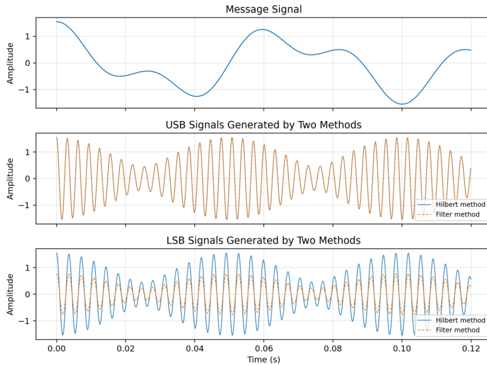
Fig. 7.5. Time-domain comparison of filter-method and Hilbert-method SSB signals.
